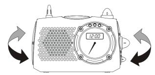
**FM, TV, WEATHER BAND** – The telescopic antenna on the top of the unit is for these bands only. If reception is weak, adjust the length of the antenna.
